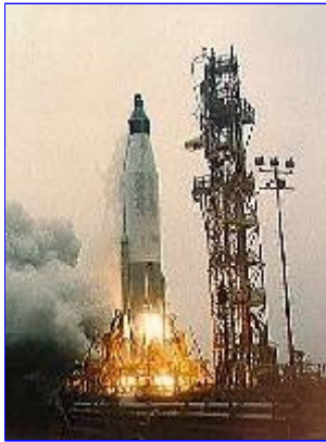
MA-1, launched like Big Joe without an escape tower, is seen 60 seconds before its demise. NASA Photo
