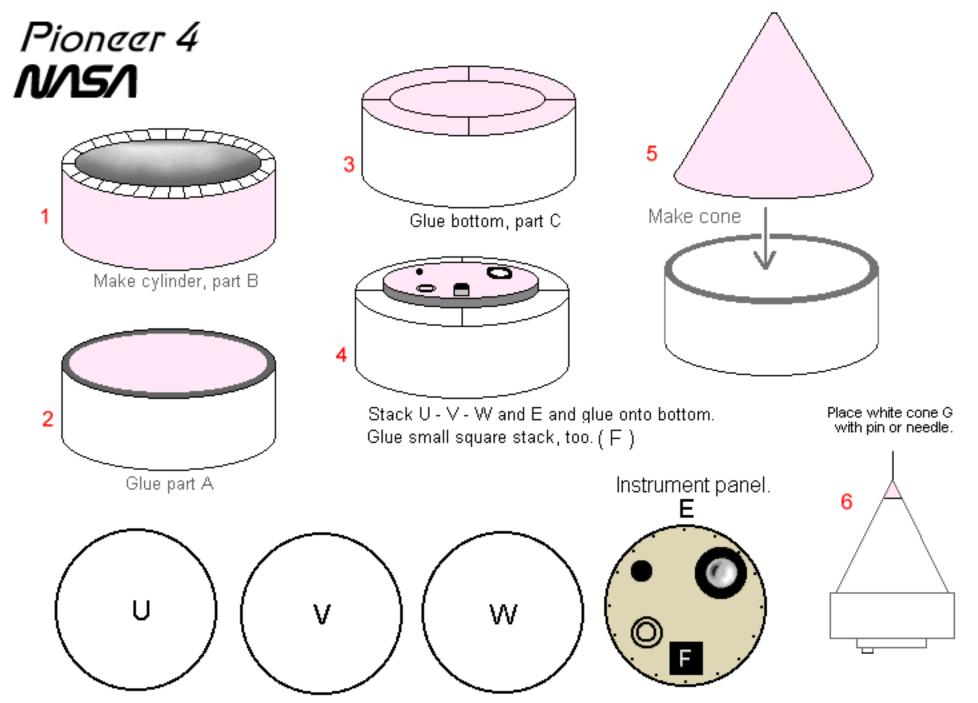
Stack these 4 circles and paint sides black. Make at least 4 mm thick. Cut out more circles if necessary to obtain thickness needed.
