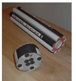
7. Glue Aft Bulkhead Mount on cardstock (Part 7D) to opposite (inner) side of gray area on S-1B Engine Section Inner Skin (Part 7A).
