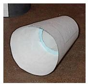
29. Cut out Spacecraft LM Adapter (SLA) (Part 12A). Trace outline to make SLA Inner Skin on a blank sheet of paper. Overlap two parts about 50%, then roll into a truncated cone. SLA housed Grumman-built Lunar Module, but was empty during Apollo 7 mission. The SLA and its contents and the CSM comprised the Saturn rocket's "payload".
